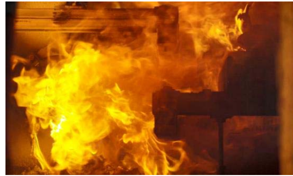
2. Assembly is exposed to fire test.
