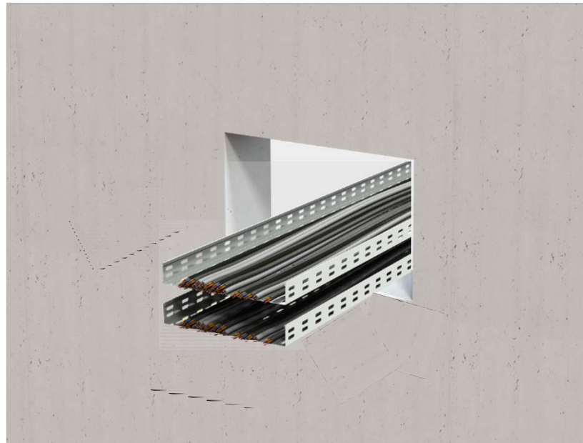
Cable trays through 2 hour fire-rated concrete wall assembly
