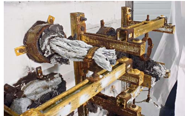
4. Assembly results after hose stream.
