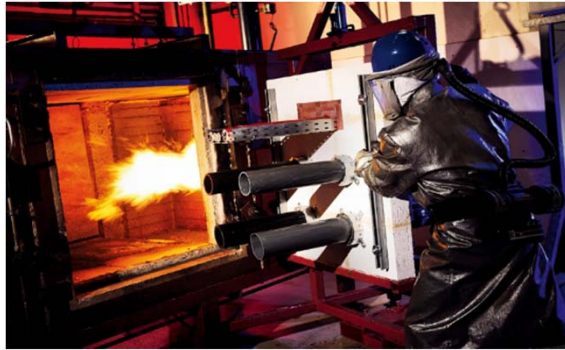
1. Assembly is placed on furnace.
