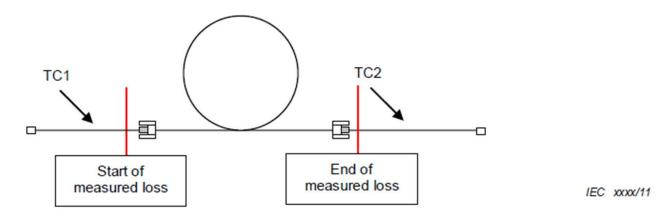
Figure 3 – Configuration A – Start and end of measured losses in reference test method
