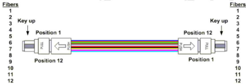
Figure 11 – Type-B:1-1 array patch cord and array cable (key-up to key-up)
