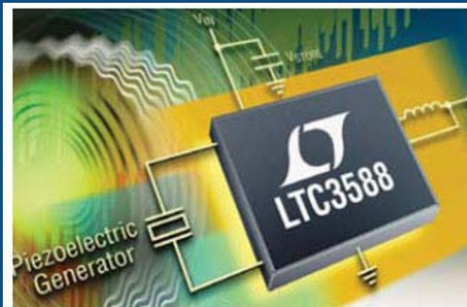
Fig. 3. The LTC3588-1 employs a high-efficiency buck converter to harvest ambient vibrational energy via piezoelectric transducers, and then convert it to a well-regulated output for use by other components.
